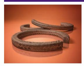
Plaited square from unbleached, ramie fibers, C-68 is designed to be a cold water centrifugal pump packing where the economy of flax, without the characteristic swell of flax, is desired. It is impregnated with petroleum base oils and waxes and contains no tallow. C-68 is suitable for use in fresh or salt water, as well as cold oils.
