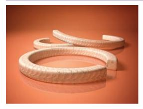
C-49 is a very popular, general service packing for rotating, reciprocating or valve service. It is made from a special glass yarn that is braided with the strong, interlock pattern, saturated with PTFE, then treated with a special blocking wax and break-in oil. C-49 performs extremely well in the critical performance areas of minimum gland adjustments, low shaft wear, low leak rate, and long life. C-49 is not recommended in steam service.
