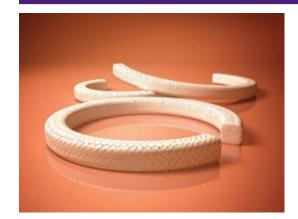
VX-1 is made of 100% white PTFE yarns, braided square using the interlock construction. It contains no impregnant, has no lubricant, and has no finish treatment. VX-1 is designed for use in valves, but can be used in other low speed services.
