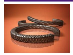
Carbon fiber is coated with PTFE suspensoid; braided into a strong, long wearing, interlock construction, then impregnated with PTFE. Applications for C-44 include pumps, valves, expansion joints, agitators and mixers. C-44 is recommended as a general service packing, but it can also handle corrosive service.
