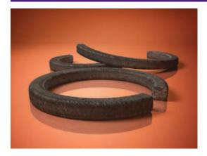
C-51 is an interlock braided, synthetic-yarn packing that utilizes a special wax and graphite lubrication system, plus a proprietary blocking agent to impart exceptionally low friction and excellent sealability properties. C-51 handles a wide range of chemicals and is recommended for centrifugal pumps, reciprocating pumps, or valves handling mild acids and alkalines, hot and cold water, alcohol, brine, or petroleum.
