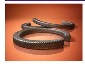
100% GFO fiber packing. GFO fiber, a patented nonasbestos fiber designed specifically for use in compression packing, is braided into a square interlock pump and valve packing. A low coefficient of friction, combined with good thermal conductivity, allows it to be used in a wide range of applications such as petroleum and synthetic oils, acids, alkalis, solvents, steam, water, or in air dry gas service.
