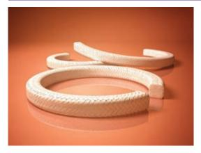
Manufactured with an Interlock braid style C-24 is an FDA approved pure white pump packing with thermal conductivity that is much greater than that of traditional PTFE packing materials. C-24 excels in fine paper bleaching applications and can be used in all types of equipment such as pumps, mixers and agitators while maintaining an extended service life rivaling that of other PTFE packing products.
