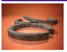
Carbon yarns are treated with graphite lubricant, braided into a tough, interlock pattern with a final graphite treatment to create this very popular packing. C-45 is a very economically priced packing suitable for an extremely wide range of centrifugal pump applications.
