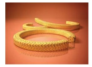
Constructed for strength using PTFE treated, Kevlar® fiber yarns, this square braided interlock packing is treated with a high temperature break-in lubricant. Designed to be used in centrifugal pumps where tough abrasion resistant performance is required from a packing, C-17 is particularly effective in the paper, petroleum, steel, and chemical industries in pumps handling wood pulp, caustic paper stock, acids, pigments and dye stock, waste effluent, demineralized and boiler feedwaters.
