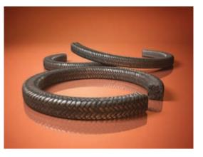
C-28 is a PTFE yarn impregnated with graphite designed specifically for use in the manufacture of compression packing, is braided into a square interlock pump and valve packing. A low coefficient of friction, combined with good thermal conductivity, allows it to be used in a wide range of applications such as petroleum and synthetic oils, acids, alkalis, solvents, steam, water, or in air dry gas service.
